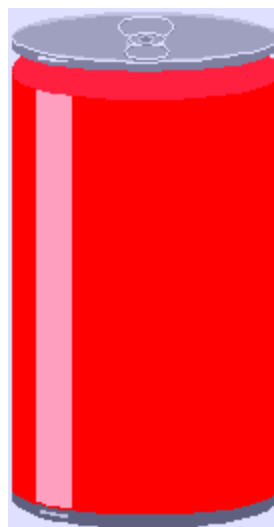
Figure 6. Spheroidality Strengthens Can's Load Bearing Capacity.
